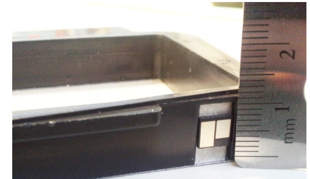
MQG Chip during relocation process. Measuring to be accurate.
