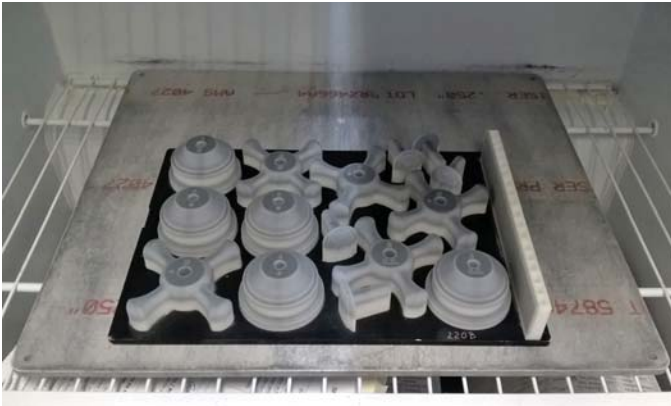
Build plate with parts attached placed on a metal plate in a freezer
