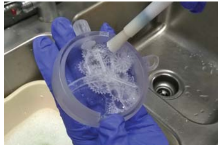
Fresh tub of soapy hot water with light brushing of part if needed
