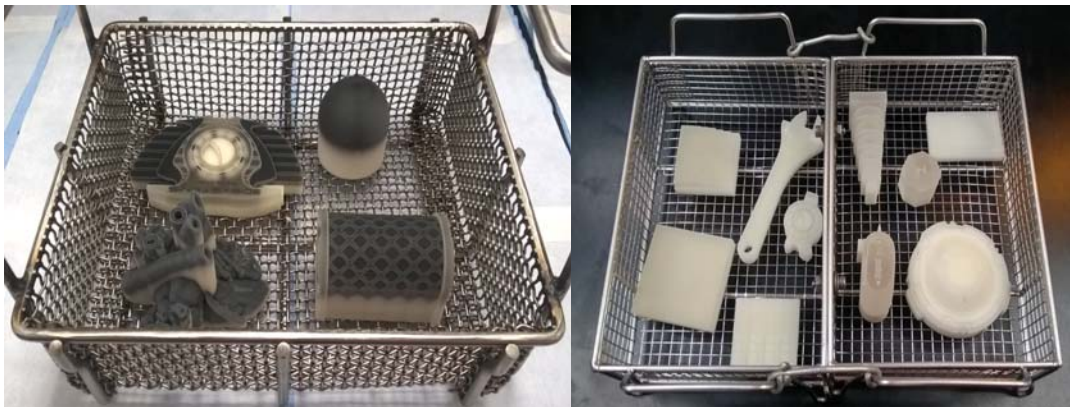
Metal baskets used to carry multiple MJP parts during post processing
