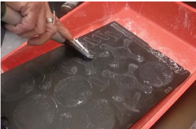
Scrape any excess support off the platform
