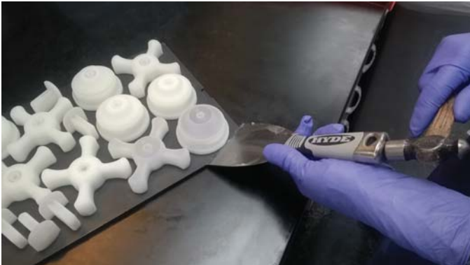
If needed, lightly tap the base of the part with a putty knife
