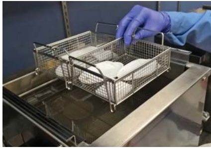
Parts placed in either EasyClean fine wax removal system or into the ultrasonic bath
