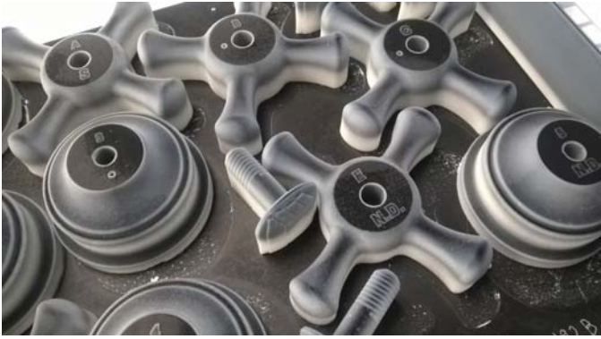
Parts typically fall free from the build plate after freezing
