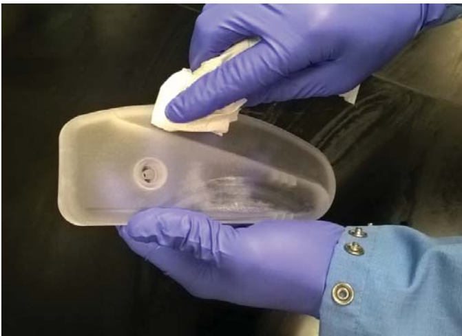
Wipe off any remaining support material with a paper towel
