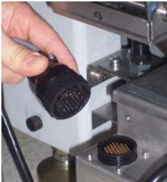
Figure 3. I/O Connector with Cable
