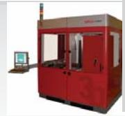
Laser position accuracy on the image plane is  $\pm 25\mu\text{m}$  average error over each image plane. The laser position resolution on each image plane is  $10\mu\text{m}$  or greater. The scanners generate a beam speed on each image plane ranging from 0 mm/sec up to 5000 mm/sec, while positioning the beam at  $\pm 25\mu\text{m}$  accuracy. It is capable of speeds up to 15,000 mm/sec at  $\pm 100\mu\text{m}$  accuracy.
