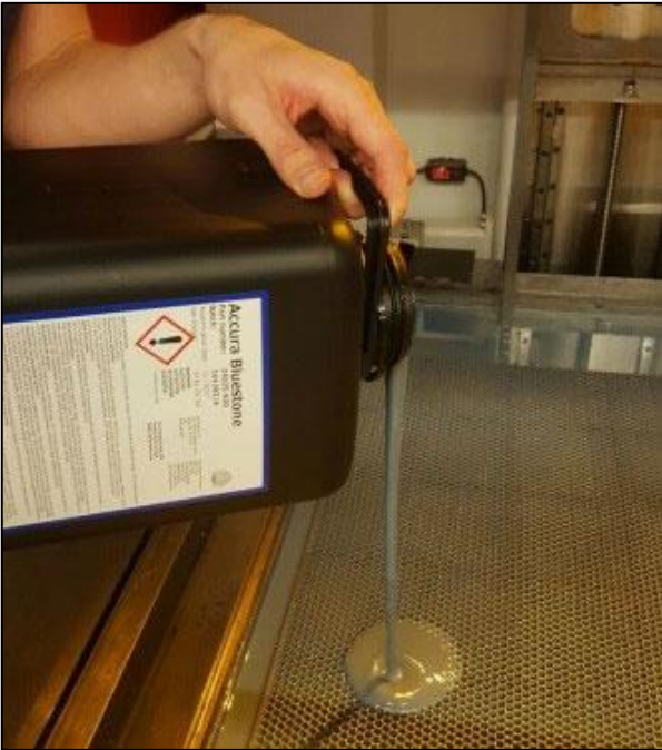
Fig. 1 – ProX 800 pictured, demonstrating an ideal place to pour resin into the MDM/RDM
