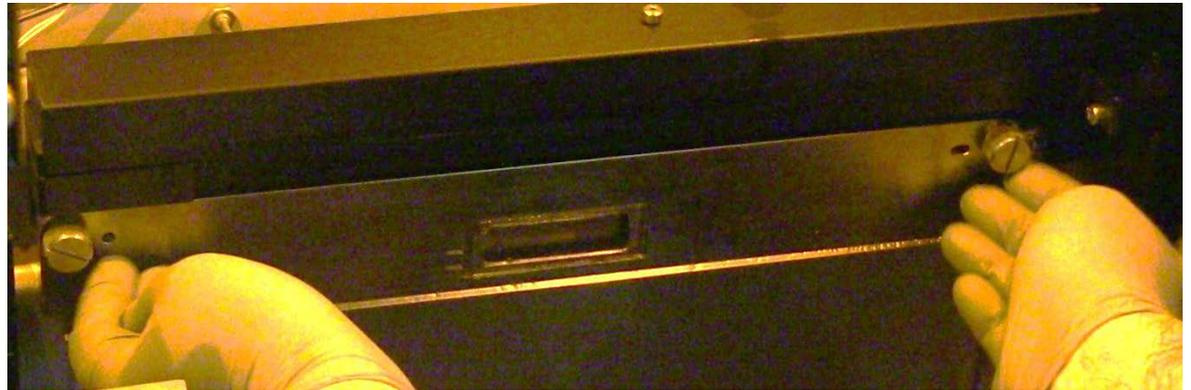
4. Disconnect the umbilical cable from the material cart. To do this, lower the latch on the connector and pull the umbilical cable out. The cable will hang close to the connector. Ensure that the cable is not damaged in the course of removing the tray and cart.
