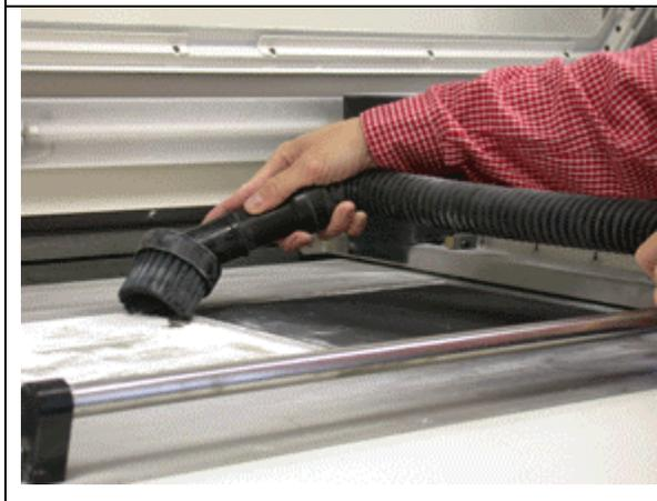
2. To prevent material contamination vacuum off any remaining powder from the feed and build plates, and the top deck.
