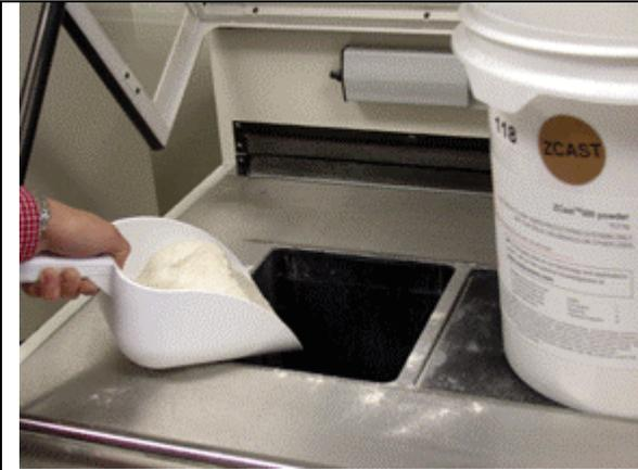
10. Lower the feed piston and fill the feed envelope with ZCast powder. You will need approximately 22 kg, or one and a half buckets of ZCast to fill the feed box.
