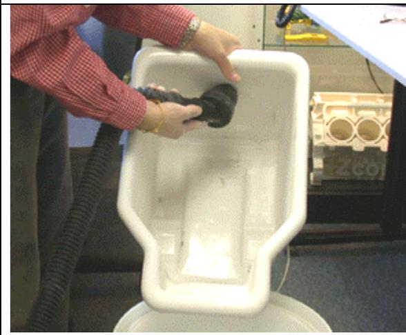
4. To prevent any material contamination, vacuum any remaining powder in the Overflow Bin.
