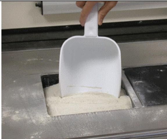
11. Use the scoop to remove any air pockets in the powder.
